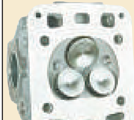
▲ EXHAUST and inlet valves are opened and closed by individual rockers. These rockers are moved by a single camshaft (see below)
