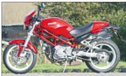
TRELLIS frame and twin pipes are traditional Ducati
