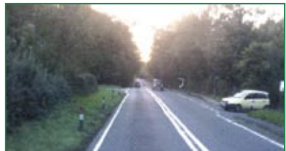
A27 Eastbourne to Lewes westbound. Poor junction score: staggered cross roads without turning lanes
